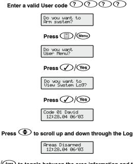
Press (h)/(Area) to toggle between the area information and the time/date Press (h)/(Part) to display zone text (where applicable)
